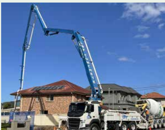
Figure 15: Concrete boom-pump operation requires approval when operating on and/or above a road .
